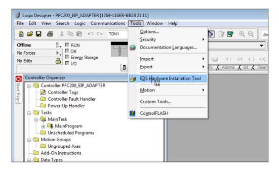
Opening the EDS Hardware Installation Tool will bring up the Rockwell Automation EDS Wizard. Select the Next > button to begin the setup process.
